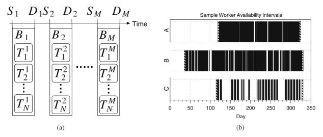
Fig. 1 Graphic depiction of tasks and batches in the low latency computing model, and three example workers with their availability intervals. a Batch diagram. b Availability intervals and worker lifespan
